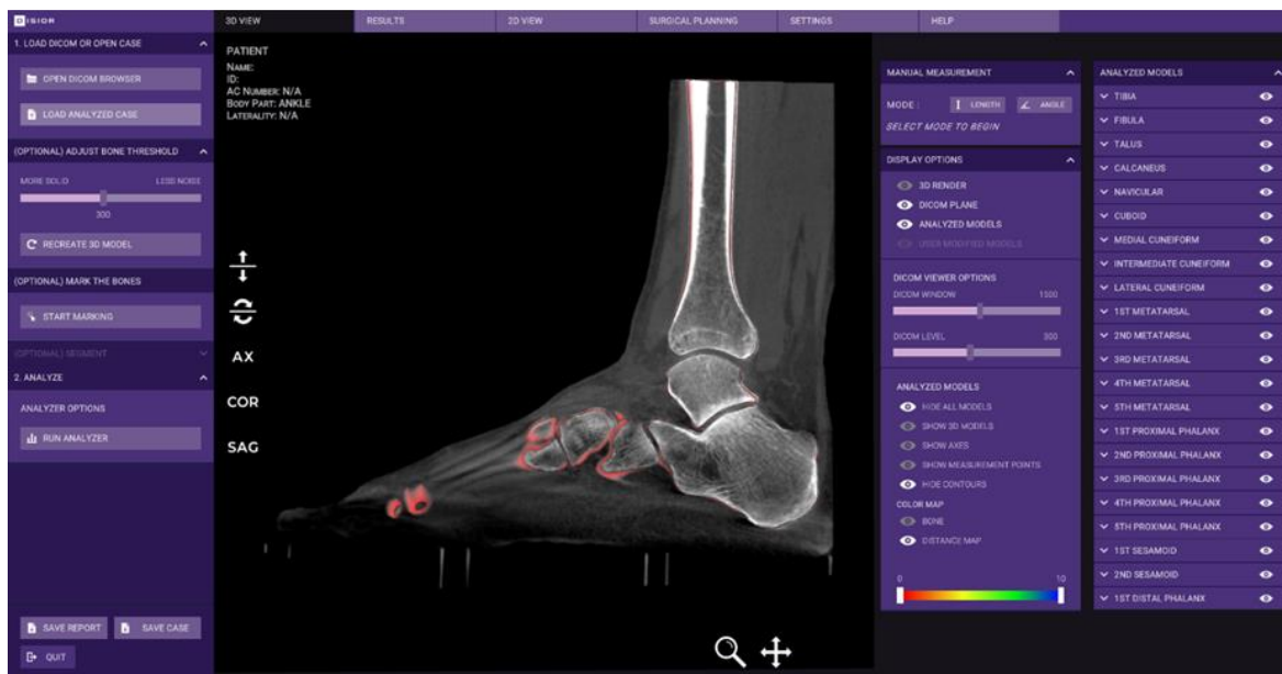
Image 14 Fusion images can be created to check the conformity of the 3D model to the original DICOM images series.
