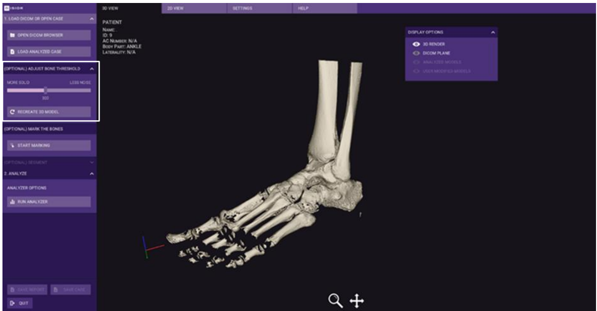
Image 3 You can change the threshold of the render by moving the 'BONE THRESHOLD' slider or typing a number and clicking 'RECREATE 3D MODEL'. Lower numbers include more data (more solid) and higher numbers include less data (less noise).
